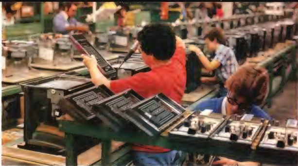
Intelligent cooking: in Iowa, an Amana Refrigeration worker installs memory and related circuits in the control panel of a microwave oven
